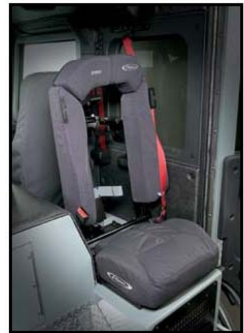
View of SCBA holder installed in rear facing Pierce PS6 seat.
